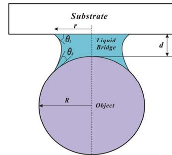
Figure 1: Illustration of a typical capillary microgripper.
