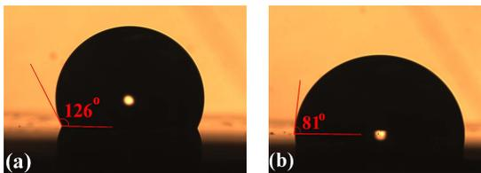
Figure 6: Contact angle change at different applied voltages
