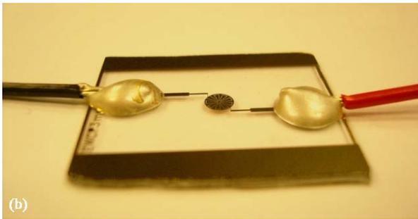
Figure 5: (a) the microscopic picture of the fabricated electrodes. (b) Picture of the fabricated microgripper.
