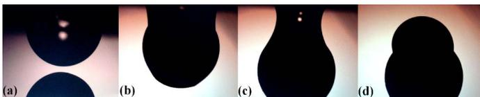
Figure 10: Microscopic pictures of the four steps of pick-up and release of a micro glass beads using the capillary micro gripper. (a) the gripper approaches object ( $V=28\text{V}$ ); (b) the object is picked at a high voltage ( $V=28\text{V}$ ); (c) the liquid bridge is elongated due to the reduction of applied voltage; (d) the object is released at a low voltage ( $V=8\text{V}$ , release voltage).
